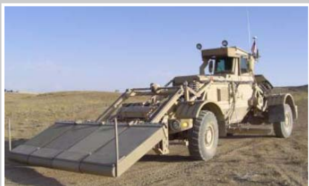
To detect buried IEDs, JIEDDO spent $33.1 million on the Husky Mounted Detection System.
